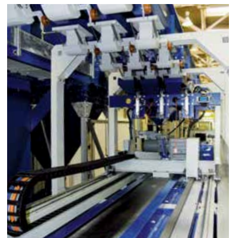
Automated blasting agent alternating system for 3 media
