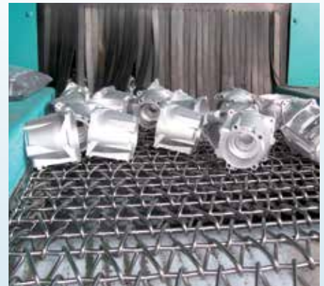
Grid belt blasting system of the model series CWB
