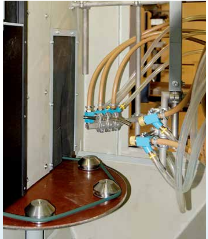
Interior view of the blasting chamber. Oscillating and stationary nozzles
