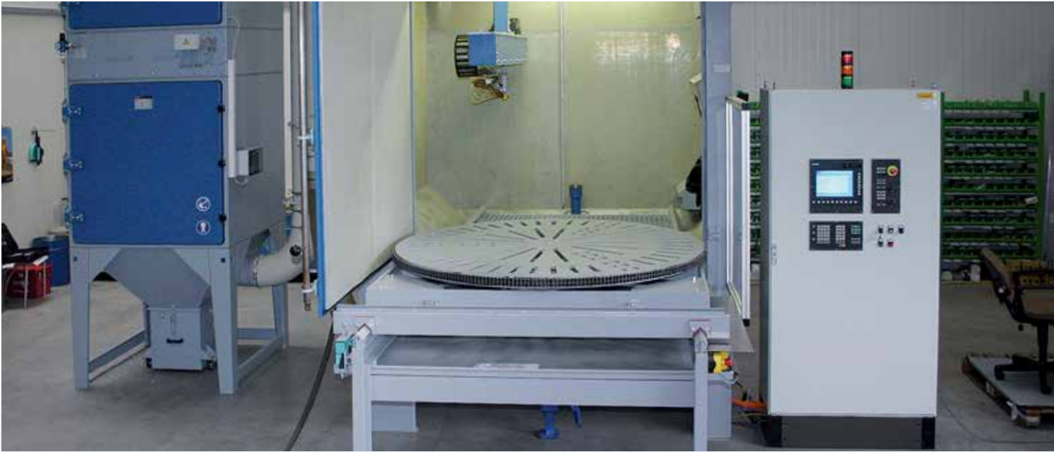
4 axle CNC universal blasting system with retractable rotary table and manual blasting position.
