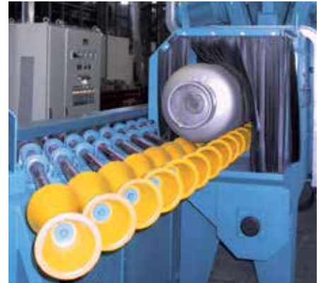
Bottle blasting system of the model series RBC
