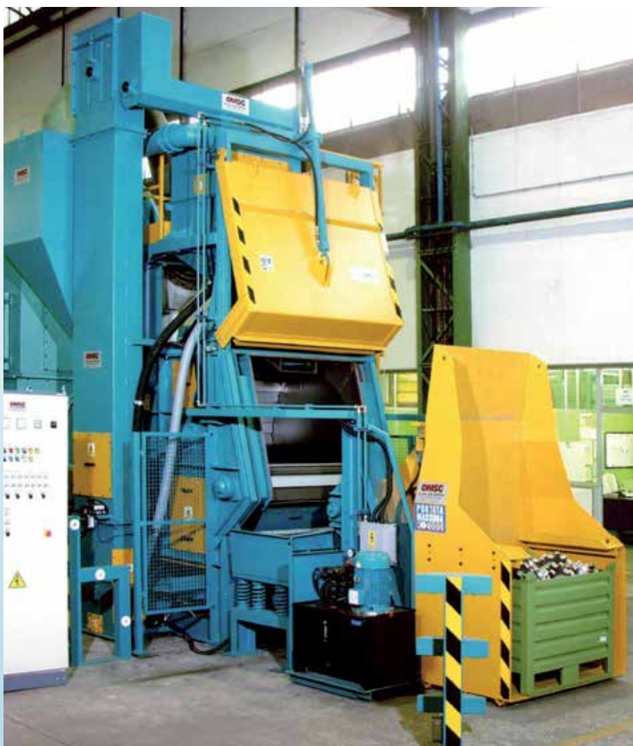
Standard steel tumbblast system with loading device (Skip) and vibro conveyor
