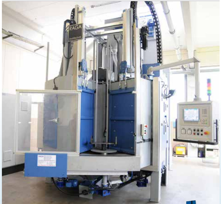
Combined blasting wheel pressure blasting system for hollow bodies with state-of-the-art control/safety technology and robot integration
