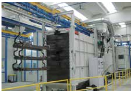
Tunnelblast 10x25 with Power & Free conveyor system.
