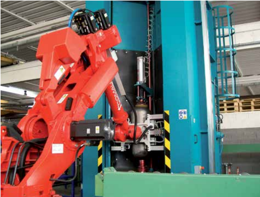
Boiler blasting system with robot feeding
