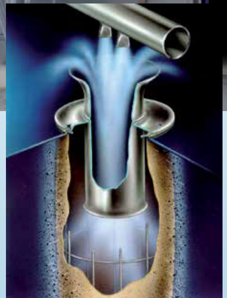
Jet cartridges cleaning principle
