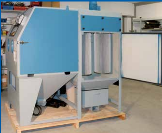
Compact 4+ view filter system with 2 filter cartridges
