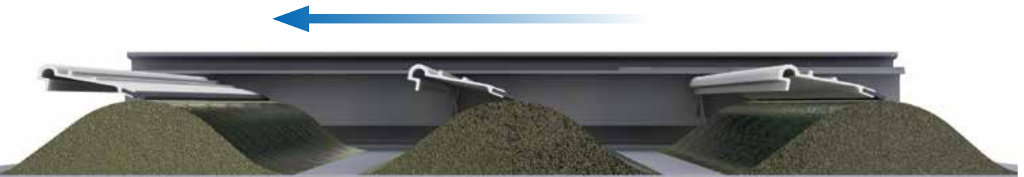
During the return stroke, the push conveyor slats slide over the blasting agent
