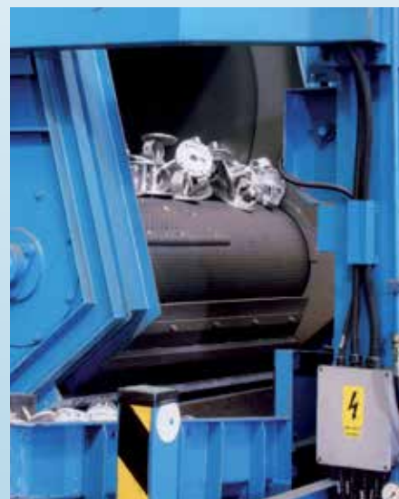
Rubber conveyor belt during unloading on the vibro conveyor
