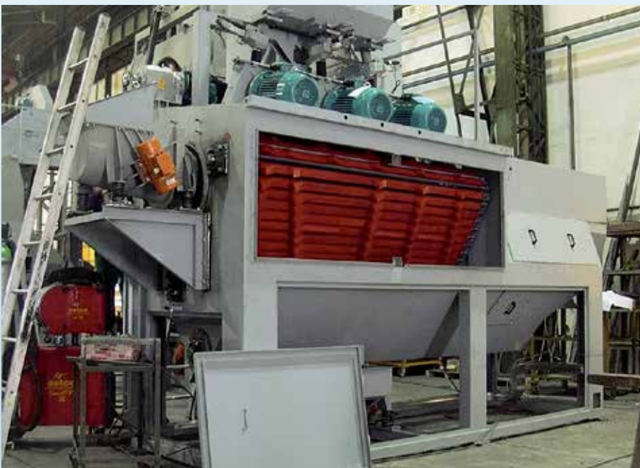
Assembling of a pass-through tumblast system of the model series Rotoflow 200
